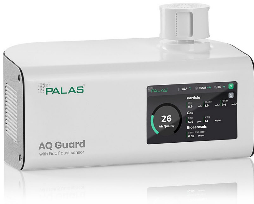
Fig. 1: AQ Guard AQ Guard is currently the most advanced compact aerosol spectrometer for determining pollution by particulates in indoor air. Using the same measurement system and sophisticated algorithms as the EN 16450 certified Fidas® 200 it analyses continuously, reliably, and precisely airborne fine dust particles in the range 175 nm – 20 µm. The "ambient" version (with heated aerosol inlet) achieves precision comparable to type approved analyzers, which makes AQ Guard stand out compared to similar devices.
